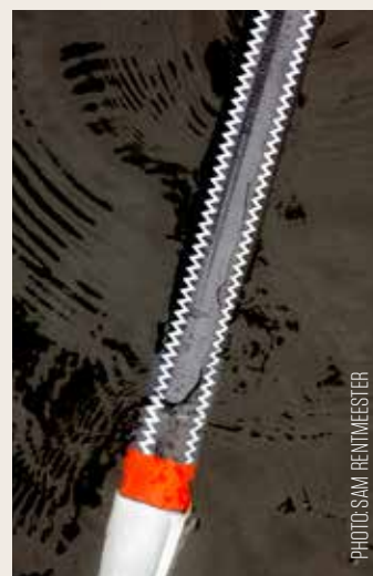
The effect of the zigzag strips is that they make the airflow along the oars turbulent, which reduces the suction effect behind the oar.
